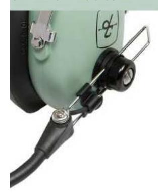
Next, <u>release the power button</u>, <u>while continuing to hold the PTT switch.</u>
